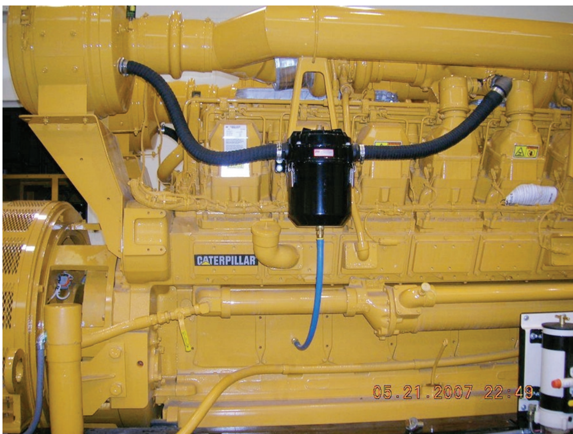
“High” mount position depicted on a CAT 3516 (ref Note 3 below)
